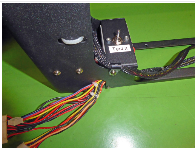
Fig. 8: X-Bearing Friction Tester mounted into the JGaurora tower
