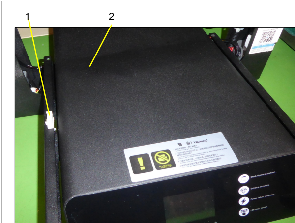
Fig. 1: Bed removed 1: Plug to Bed disconnected (Hot glue!) 2: Free Base Unit JGaurora
