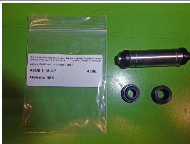
Fig. 8: High Standard Wiper Ring Kull-Laube AG, CH
